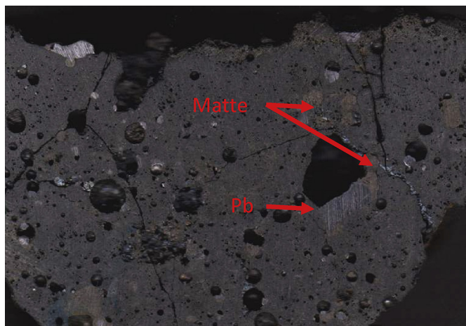
Fig. 16. Cross-section of SL1 slag. Numerous metallic lead and matte prills were found trapped in the slag.
