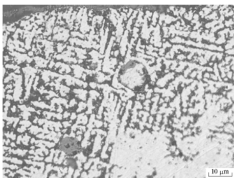
Figure 10 Bronze microstructure of M27: 970 showing \alpha + (\alpha + \delta) dendrites (unetched).
